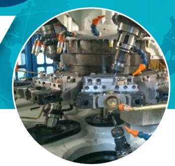
The design and and assembly of progressive metalworking equipment. The basis of its ideology is that "there is no longer just the machine—there is the automated production complex." This complex includes machines; automated loading/unloading systems; automated systems for cleaning and rinsing parts; automatic control, and automated warehouses. The use of an integrated approach makes it possible to make the production and manufacturing industry more cost-effective.
